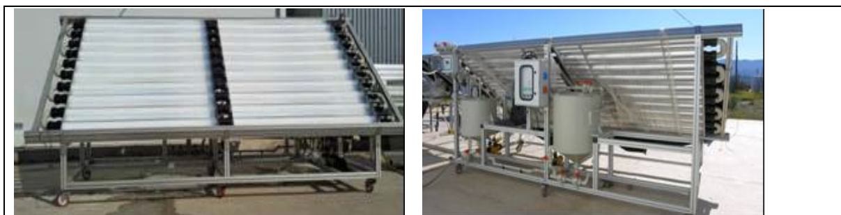
Figure 1. Picture of the CPC solar photoreactor constructed for photocatalytic disinfection of water contaminated with agricultural pathogens (PSA facilities, Spain).
