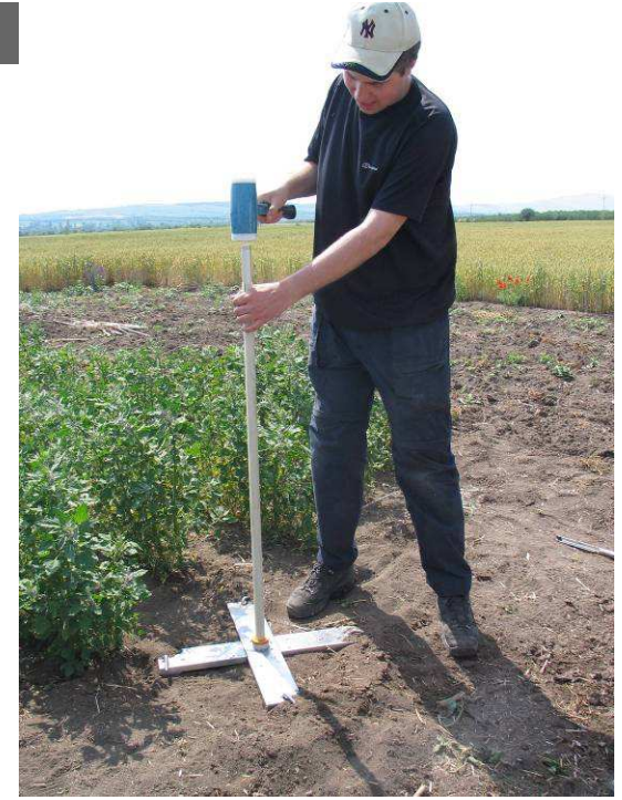
Incorporation of access tube
